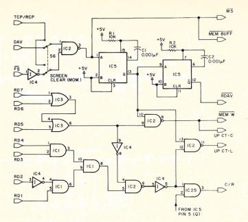
Fig. 5. Interfacing address and select lines.
